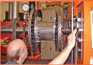
Typical Short Industry Pump Connector 12" x 14" at Maximum 0.125" Offset
